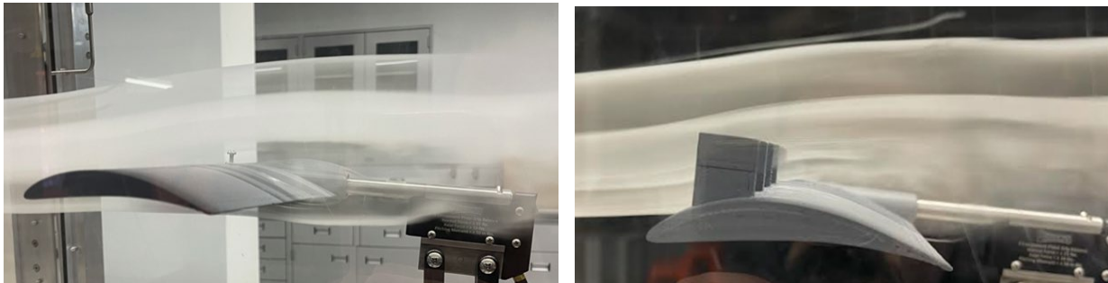
Figures 5 and 6. 5 Degree Angle of Attack Wind Tunnel Case
