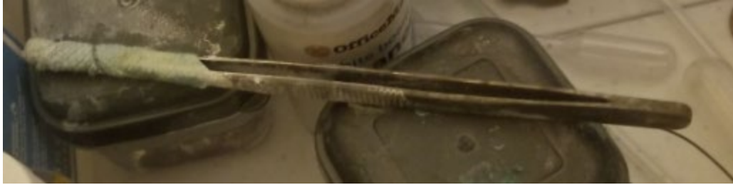
Figure 11. Homemade Anode of 316 steel tweezer and blue shop cloth
