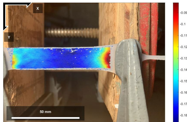
Figure 1. 2D strain field projected onto deforming sample (prototype DIC system).
