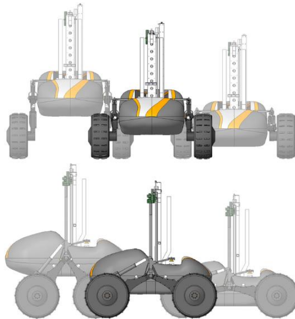
Figure 3. Varying ground clearances of the Scarab suspension design. Image sources: Reference [5].
