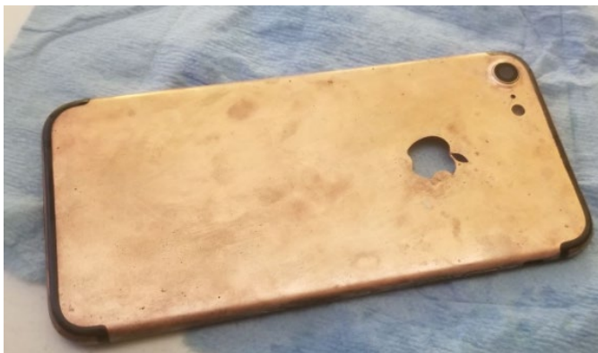
Figure 7. Acid Copper plating on iPhone 7 after alkaline dip
