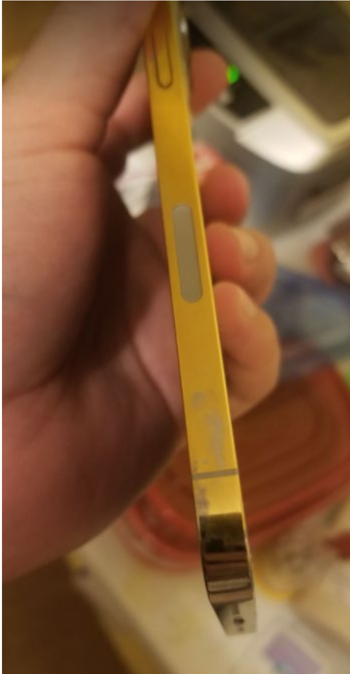
Figure 10. Poor gold plate on iPhone 12 Pro Max
