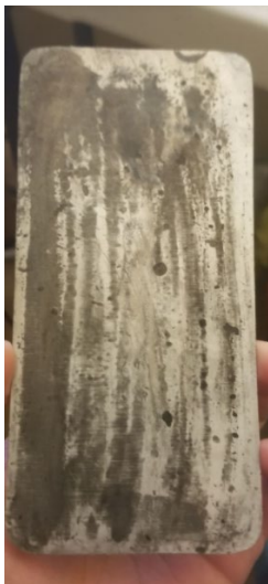
Figure 5. Poor adhesion of zincate solution on scrap aluminum
