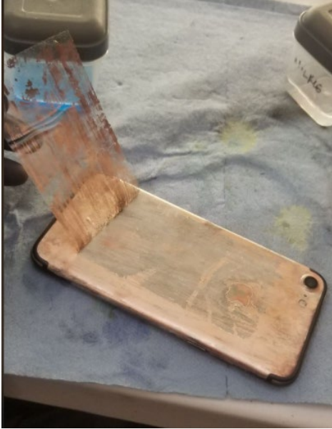
Figure 8. Adhesion test on iPhone 7
