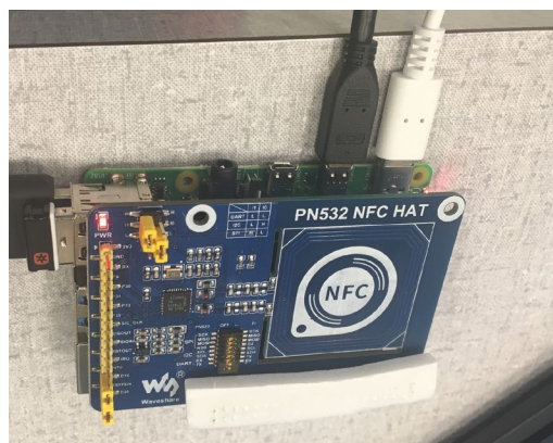
Figure 4. Photo (by author) of the hardware (NFC Hat installed on top of Raspberry Pi)
