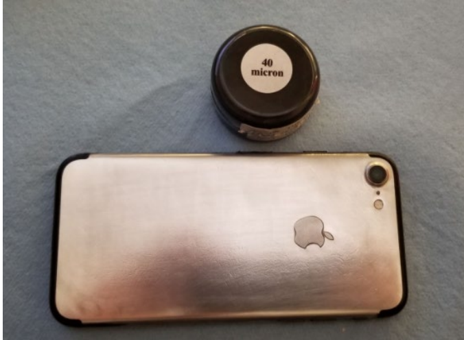
Figure 3. iPhone 7 Polished to 40 micron (325 Grit)
