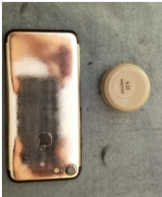
Figure 4. iPhone 7 Polished to .25 micron (100,000 Grit)
