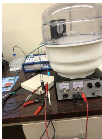
Figure 4. Solid state set-up. Gold-plated electrode with functionalized CNTs (left). Enclosed chamber for detecting the cocaine (right).
