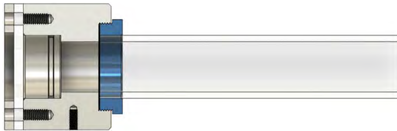
Figure 2. Section view of vortex tube.
