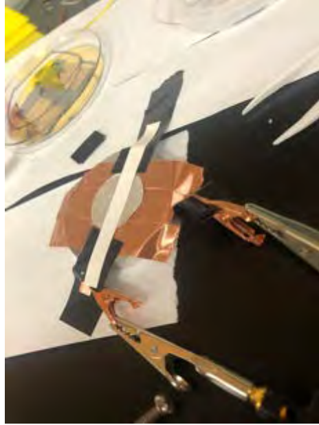
Figure 4. Finalized template attached to copper tape. Initial monitor voltage response related to physical pressure applied to template.
