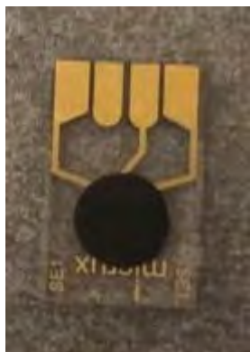
Figure 4. Solid state set-up. Gold-plated electrode with functionalized CNTs (left). Enclosed chamber for detecting the cocaine (right).
