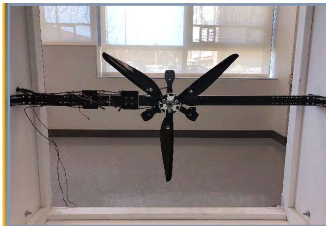
Image 1: Set up of Kent State University's eVTOL Propulsion Test Stand.
