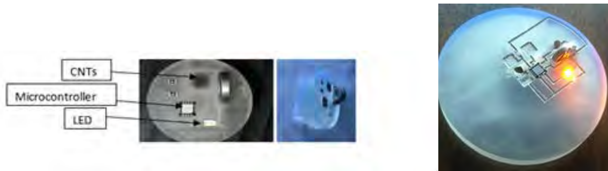
Figure 1. Stereolithography printed substrate for creating wearable sensors.
