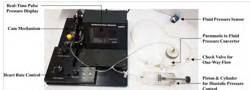
Figure 1. System developed to create fluid pressure human pulse waveforms.
