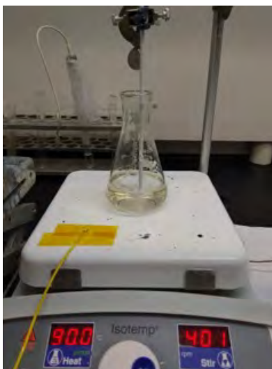
Figure 1. Nylon-11 solution prepared by dissolving nylon-11 pellets in formic acid at a temperature of 90°C.
