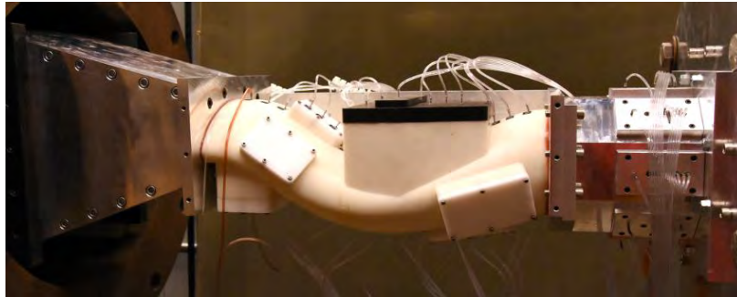
Figure 1. Side view of Offset Diffuser Facility.
