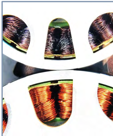
Image 3: Overexposed photograph showing charred coils (top) versus normal coils (bottom) of the 7215XF motor.
