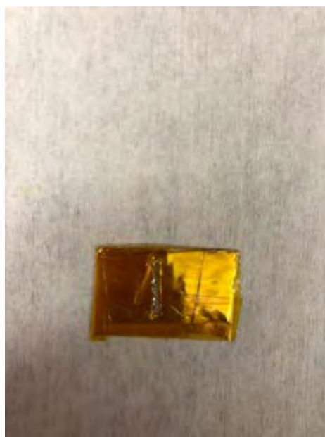
Figure 3. Nylon-11 attached to aluminum sheet, encased in tape. The slit in the middle allowed for chemical etching.
