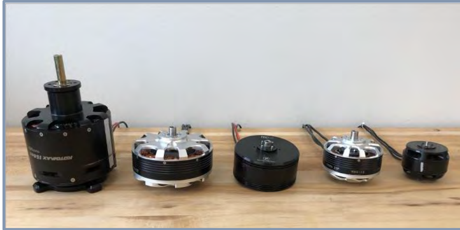
Image 2: Comparison of motor sizes (left to right: RotoMax, 10218XF, P80, 7215XF, U7).
