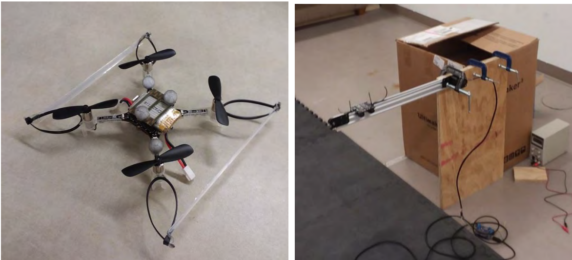
Figure 9. Crazyflie 2.0 quadrotor used for test flights (left), linear actuator setup for collecting disturbance response data (right)
