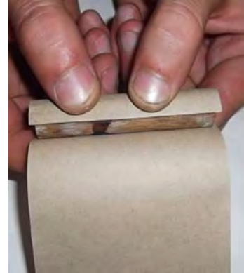
Figure 4. Kraft paper wrapped around a dowel rod to make a pliable but strong fuel casing
