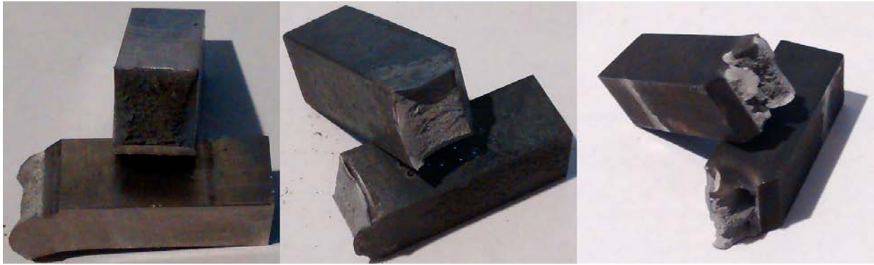
Image 2. Charpy test samples. From left to right: Control, Normalized, and Hardened
